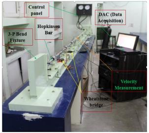
Fig.2 Actual photograph of three points bend setup for Modified Hopkinson Bar
